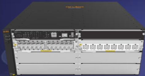
Aruba 5406R zl2 Switch
