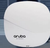
BLE-enabled Aruba APs
