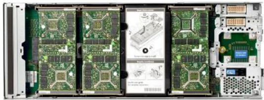
Synergy 480 Multi-MXM Graphics Expansion Module
