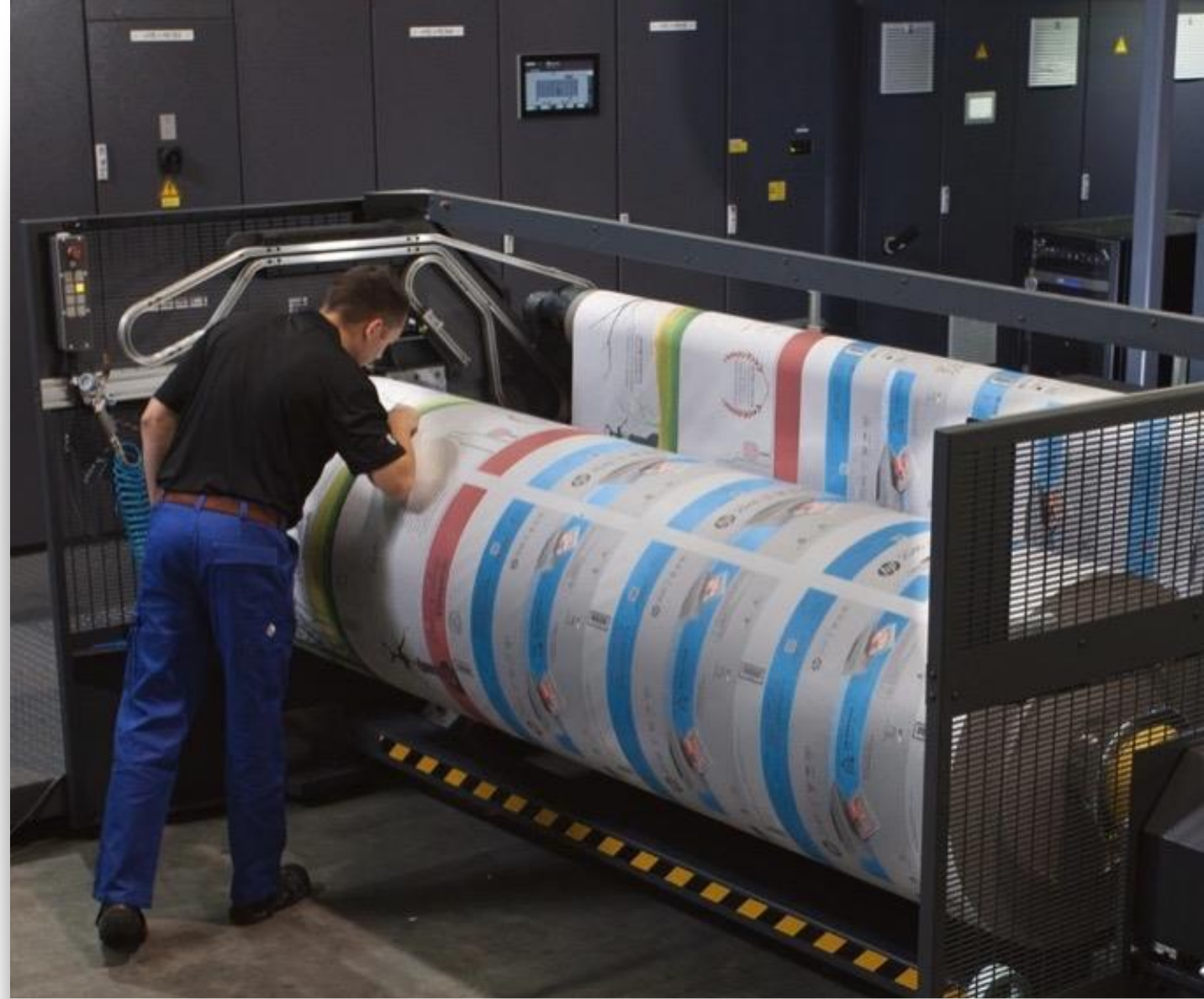
2.8 meter wide Thermal Inkjet digital printing
