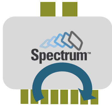
Downlink to Downlink Full Cut-Through
