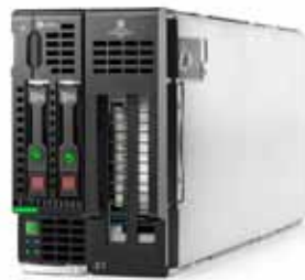
WS460c Gen9 Graphics Server blade with Expansion 8 per 10U enclosure
